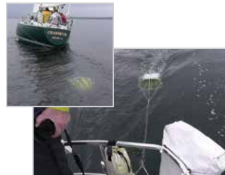
Steering with a Galerider drogue deployed astern.
