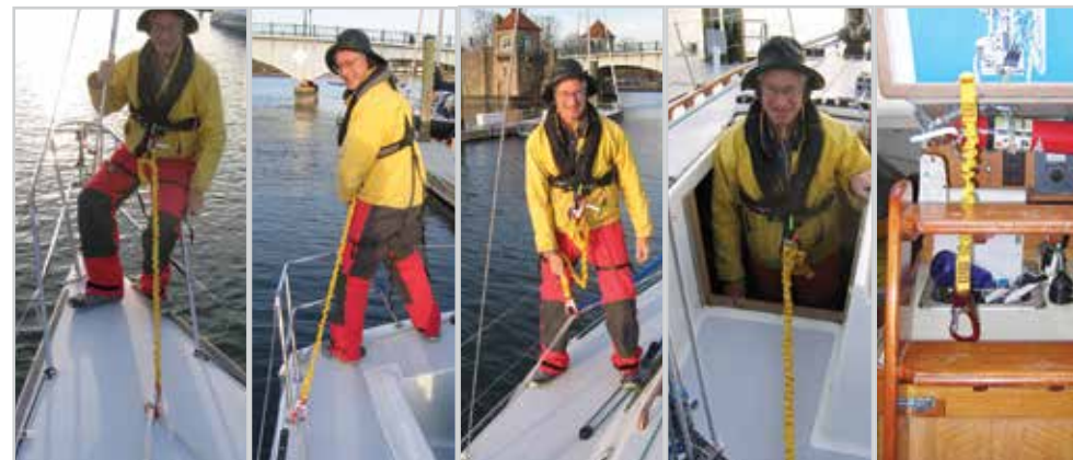
Photo 1: Jackline terminates center of foredeck- tether fetches up before crew drops lower than rail- no dragging in the water. Photo 2: Jackline terminates before reaching stern- tether fetches up before crew can go over stern or drag aft of transom. Photo 3: “Walk Like a Man”—straddle the tether and pull up on jackline for stability. Photo 4: Always remained tethered as you go up/down companionway. Photo 5: Leave tether hanging after feet are on cabin sole; hook up before ascending.
